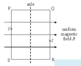
A coil, mounted on an axle, has its plane parallel to the flux lines of a uniform magnetic field *B*, asshown. When a current / is switched on, and before the coil is allowed to move,
