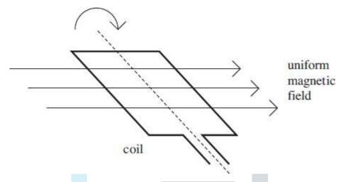
When the coil is rotated at a constant rate, an alternating emf  $\varepsilon$  is induced in it. The variation of emf  $\varepsilon$ , in volts, with time t, in seconds, is given by
