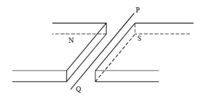
A wire lies perpendicularly across a horizontal uniform magnetic field of flux density  $20 \times 10^{-3}$  T so that 0.30 m of the wire is effectively subjected to the field. If the force exerted on this length of wire due to a current in it is  $30 \times 10^{-3}$  N downward, what is the current in the wire?
