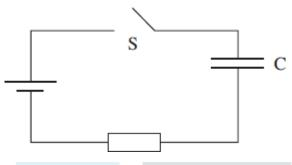
Which line, A to D, in the table gives a correct pair of graphs showing how the charge on the capacitor and the current in the circuit change with time after S is closed?
