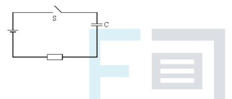
Which line, **A** to **D**, in the table gives a correct pair of graphs showing how the charge and current change with time after S is closed?
