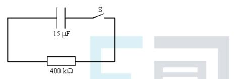
The switch S is closed at time t = 0. Which one of the following statements is correct?
