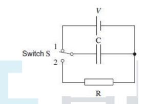
The switch is then moved quickly to position 2, allowing C to discharge through the fixed resistor V
