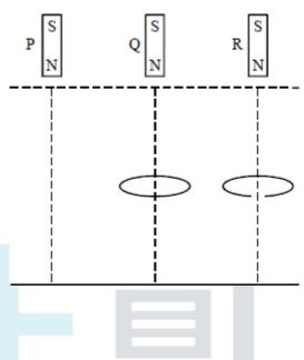
Three identical magnets P, Q and R are released simultaneously from rest and fall to the ground from the same height. P falls directly to the ground, Q falls through the centre of a thick conducting ring and R falls through a ring which is identical except for a gap cut into it. Which one of the statements below correctly describes the sequence in which the magnets reach the ground?
