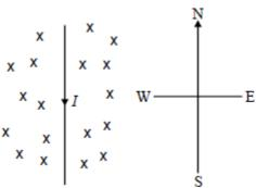
The diagram shows a wire carrying a current, *I*, in the plane of the paper and in the south direction. A magnetic field is applied perpendicularly to the paper and acts into the paper. What is the direction of the force acting on the wire?
