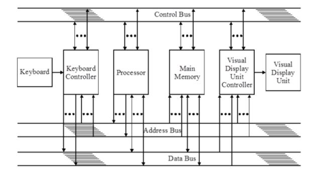
The figure above is a block diagram showing the bus architecture of a typical microcomputer. A device controller is a hardware unit which is attached to the bus system of the computer to provide a hardware interface between a computer and a device such as a keyboard.
