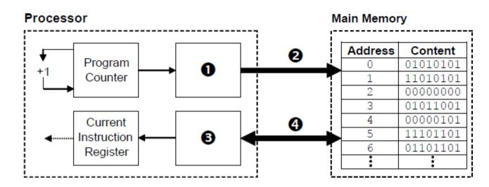
(a) Name the components that are labelled with the numbers 1 to 4. In the case of register names, the full names must be stated.
