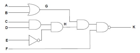
Complete the truth table for the inputs that have been given.
