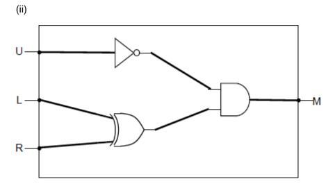
L, R connected to XOR gate; U connected to NOT gate; Output of a two input AND gate connected to M;
