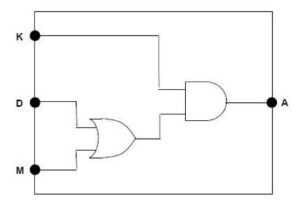
1 mark: inputs D and M connected to an OR gate;
