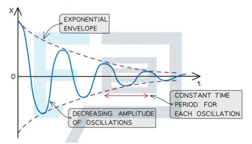
A graph for a lightly damped system consists of oscillations decreasing exponentially
