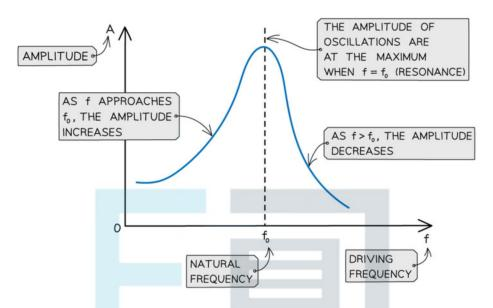
The maximum amplitude of the oscillations occurs when the driving frequency is equal to the natural frequency of the oscillator
