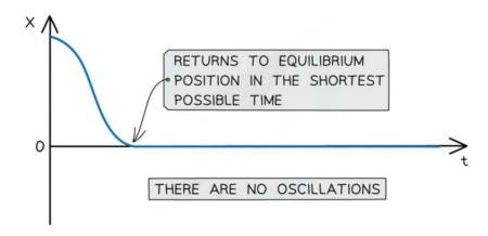
The graph for a critically damped system shows no oscillations and the displacement returns to zero in the quickest possible time
