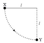
A ball of mass m, which is fixed to the end of a light string of length I, is released from rest at X. It swings in a circular path, passing through the lowest point Y at speed v. If the tension in the stringat Y is T, which one of the following equations represents a correct application of Newton's laws of motion to the ball at Y?
