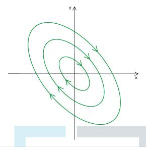
TRAJECTORIES 'ORBIT' AROUND THE ORIGIN. THEY MAY BE ELLIPTICAL OR CIRCULAR, AND MAY BE CLOCKWISE OR ANTICLOCKWISE (BUT ALL WILL EITHER BE ONE OR THE OTHER FOR ANY PARTICULAR DIFFERENTIAL EQUATION).
