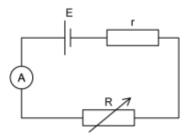
The load resistance *R* is varied such that a graph of the quantity *IR* can be plotted against the current *I*, using readings from the ammeter.
