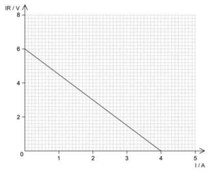
Which row, **A** to **D**, gives the correct values for the emf *E* of the cell, its internal resistance r and the powerdissipated in the load resistance when the current is 1.5 A,  $P_{1.5}$ ?
