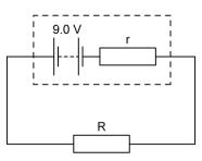
A charge of 240 C through the resistor in two minutes. The power dissipated in the resistor as a result is 1440 J. What is the internal resistance *r* of the battery?
