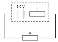
A charge of 240 C through the resistor in two minutes. The power dissipated in the resistor as a result is 1440 J. What is the internal resistance r of the battery?
