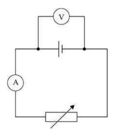
When the resistance of the variable resistor is 10  $\Omega$  the voltmeter reads 10 V and the ammeter reads 1.0 A.
