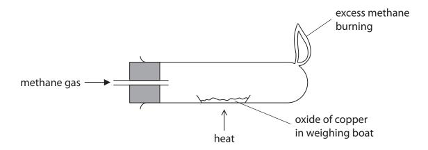
The oxide of copper is heated until the reaction is complete.
