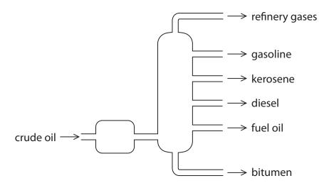
(a) (i) Describe how crude oil is separated into fractions in the fractionating column.
