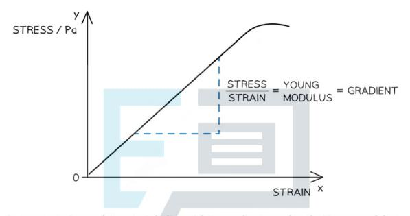
A stress-strain graph is a straight line with its gradient equal to the Young modulus
