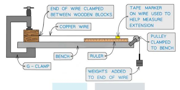
This method is an example of the procedure for varying load and measuring the extension of a copper wire. This is just one way of measuring the relationship between them.
