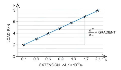
4. Multiply the gradient by the ratio of the original length and cross-sectional area of the wire to calculate the Young Modulus
