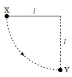
A ball of mass m, which is fixed to the end of a light string of length l, is released from rest at X. It swings in a circular path, passing through the lowest point Y at speed v. If the tension in the stringat Y is T, which one of the following equations represents a correct application of Newton s laws of motion to the ball at Y?
