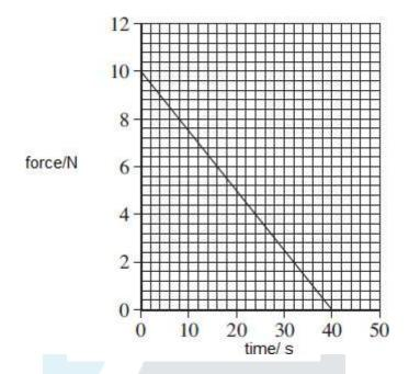
The body has a mass of 0.25 kg and is initially at rest. What is the speed of the body after 40 sassuming no other forces are acting?
