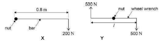
What is the minimum length /of the wrench which would be needed for him to loosen the nut?
