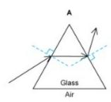
as the light passes into the glass prism initially it follows the correct direction and bends towards the normal. However, as the light passes out of the glass prism it enters a medium of lesser refractive index, so it should bend toward the normal. This is not shown in option B
