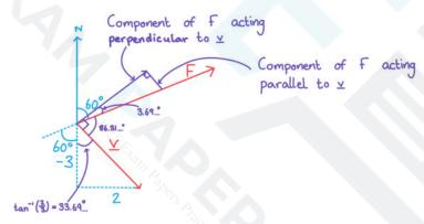
Component of F acting parallel to  $x = 10 \sin 3.69^{\circ}$
