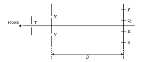
Coherent monochromatic light of wavelength  $\lambda$  emerges from the slits X and Y to form dark fringes at P, Q, R and S in a double slit apparatus. Which one of the following statements is true?
