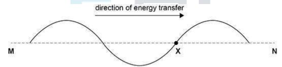
The wave has a frequency of 5.0 Hz, a wavelength of 1.0 m and an amplitude of 0.20 m.
