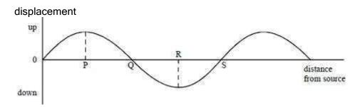
The graph shows, at a particular instant, the variation of the displacement of the particles in a transverse progressive water wave, of wavelength 4 cm, travelling from left to right. Which one of the following statements is **not** true?
