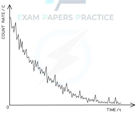
The variation of count rate over time of a sample radioactive gas. The fluctuations show the randomness of radioactive decay
