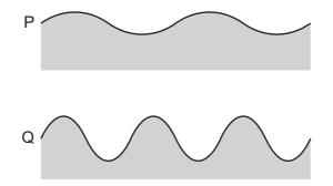
Which wave has the greater amplitude and which wave has the greater frequency?
