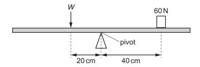
A weight *W*, placed 20 cm from the pivot, balances the beam.
