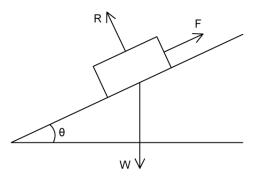
R is the normal force, W is the weight and F is friction.
