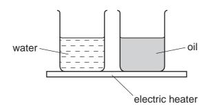
The temperature of the water and the temperature of the oil increase constantly. The rise in temperature of the oil is much greater than that of the water.
