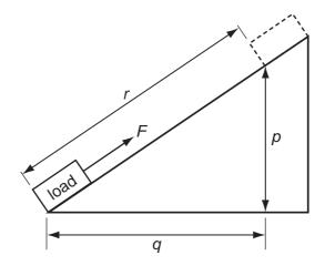
The work done by the force depends on the size of the force, and on a distance.
