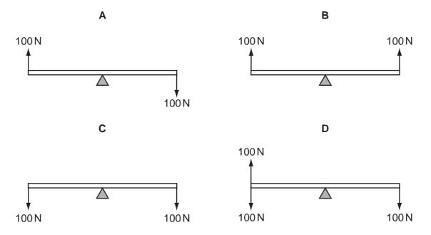
8 Which combination of forces produces a resultant force acting towards the right?
