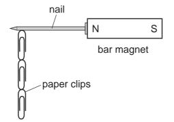
One of the nails is placed against a bar magnet and the number of paper clips which the nail can support is recorded. The bar magnet is then removed and the number of paper clips remaining attached to the nail is recorded. Each nail is tested in turn.
