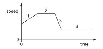
Which section of the graph shows acceleration and which section of the graph shows deceleration?
